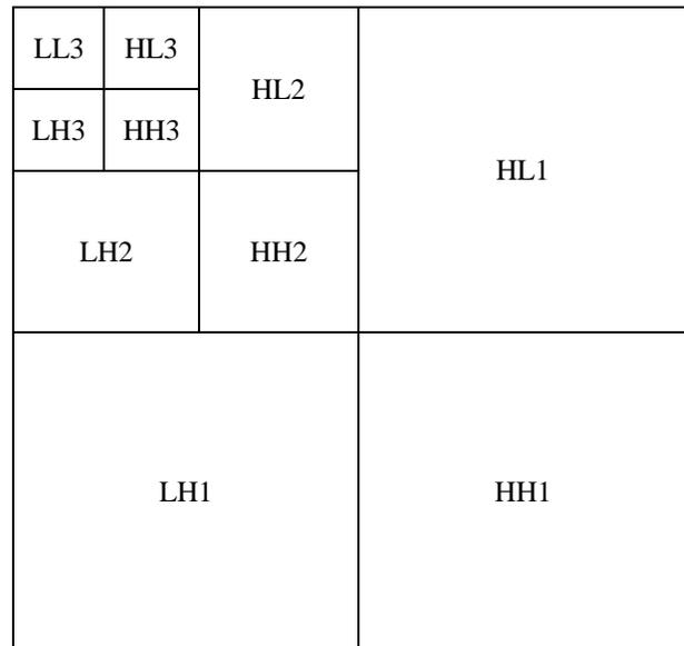
Figure1 Three level image decomposition using DWT
